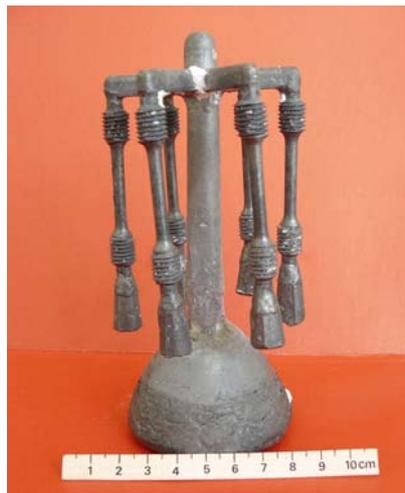
Fig. 2. Assembly of precision cast samples for tensile tests
